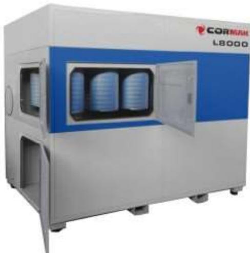
An extractor for industrial purposes. Due to the implementation of filters from a renowned Donaldson company, which are equipped with a layer of fibers from 0.2 to 0.3 micron in diameter, it is easier to filter the particles smaller than 1 micron. The extractor is perfect for draining out the smoke created as a result of cutting metals using optical fiber lasers or plasma burners.
